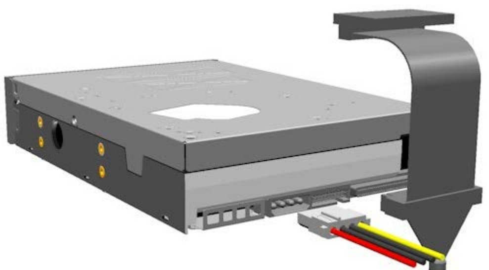
Figure 6: Connecting the cables to the tape drive
